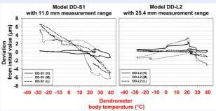
In the performed rapid test, the course of the individual measurement series did not result in simple linear correlations, but appeared to be superimposed by varying degrees of hysteresis and randomly directed effects.
