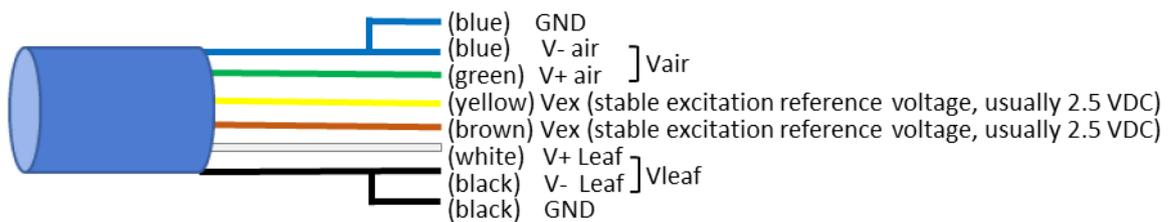
Figure A: Differential wiring
