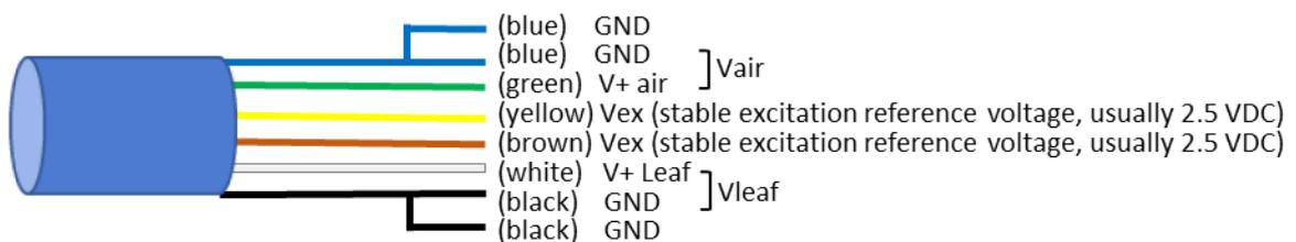
Figure B: Single-ended wiring
