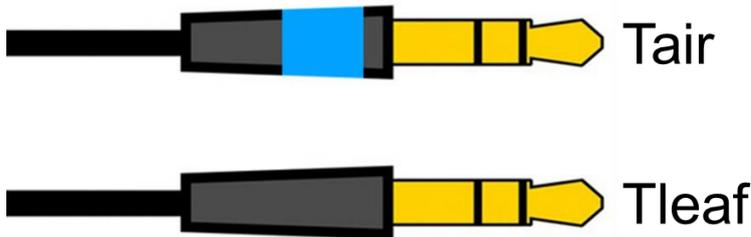
Figure C: Stereo plug connector for DL 18 logger
