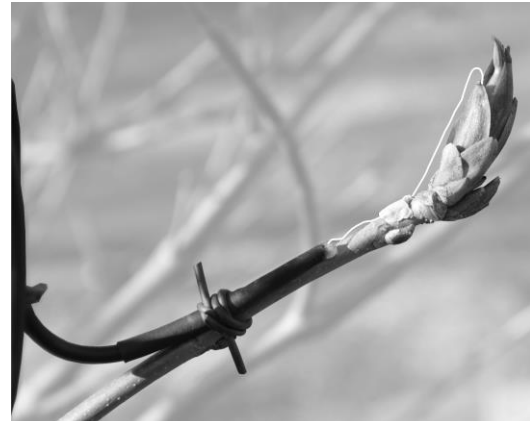
T-Tissue sensor non-invasively inserted into an opening bud.
