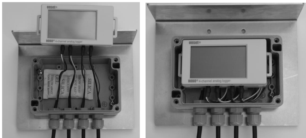
Fig. 3 Connecting dendrometers to the logger
