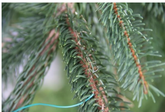
leaf temperature sensor type ΔLA-C on Norway spruce
